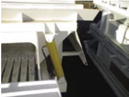
Hydraulic Side Dump Grizzly with Deflection Plate
