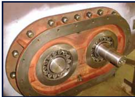
Twin shaft with 110 mm bearings
