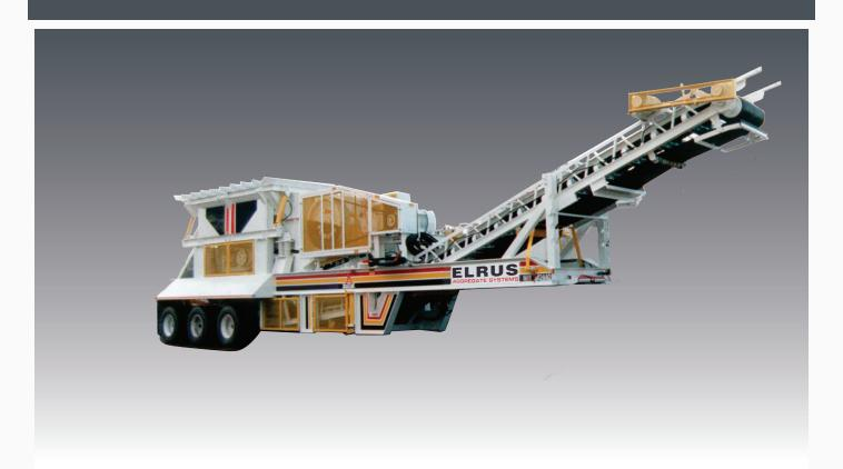
The ELRUS 2236 100 HP Primary Jaw Plant is our smaller heavy duty overhead eccentric jaw crusher. It is ideal for the contractor who needs the features of a big crusher in a smaller size. It's features are:
