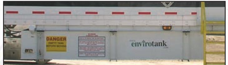
7774 liter (2050 US gal) double walled underslung generator fuel tank c/w locking filler cap and fuel level indicator
