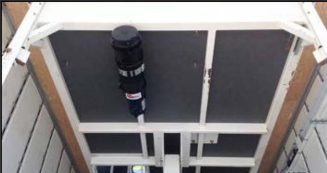
A combination air pre-cleaner with VLR air filter system removes large particles with a built in centrifugal pre-cleaner. Air is then filtered and blown in with a self contained air pump. The clean air is blown into the cab creating a positive pressure which prevents dirt from entering the cab through leaks in its doors and other spaces.
