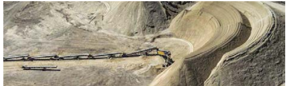
RADIAL WINDROW STOCKPIILING ACHIEVES IN-SPEC MATERIAL MIX
