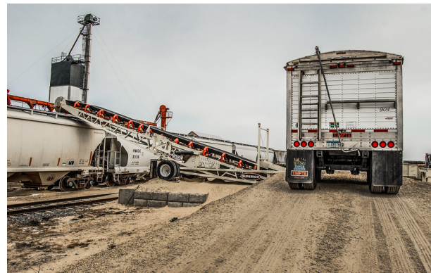
BELLY DUMP TRAILER TO RAILCARS
