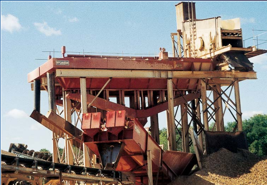
Twin 10' x 40' Sand Classifying Tank In Texas
