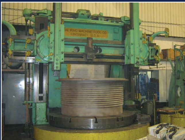
Cone Rebuilds (HP 400 Bowl on Vertical Lathe)
