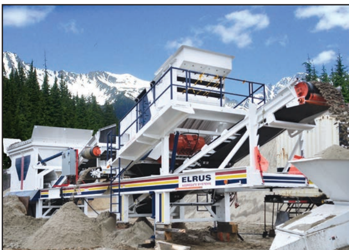
MS612 Feeder Screen Plant
