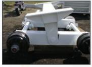
Tandem Axle Walking Beam Suspenion
