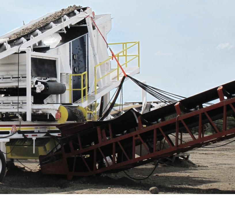
Beyond performance, the MS612 is designed for operator ease and convenience. Simplified maintenance and service allow for easy access and upkeep, while its compact size—63,626 lbs (28,860 kg) and 51' in travel length—makes it lighter and shorter than comparable models, ensuring effortless mobility and setup. Often, the MS612 can be transported across pits or even across the country without requiring disassembly or special permits.
