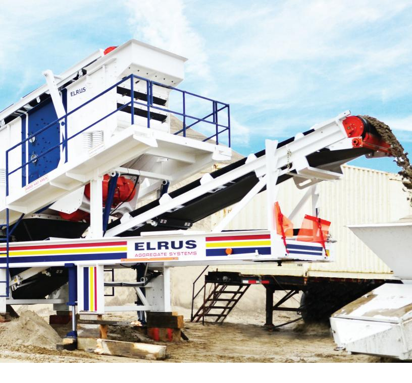
For efficient and reliable material handling, the plants are equipped with an 8' x 13' self-relieving hopper capable of holding up to 15 cubic yards. Designed for smooth operation and minimal maintenance, this feature minimizes downtime while maximizing efficiency. Additionally, the hydraulic side-dumping Grizzly, with heavy-duty adjustable bars, 4" diameter dumping cylinders, and a complete motor, pump, and controller system, provides precise control and enhances overall performance.
