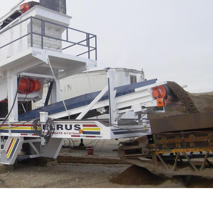
Other features include folding blocking legs for accommodating tandem jeep axles, optional full-end tension on the bottom and middle decks, and adjustable height for the overhead conveyor. With the choice of two or three cross conveyors, angled cross members on carry decks for improved stability, and hydraulic levelling for easy setup on uneven terrain, ELRUS screening equipment ensures reliable and efficient operation.
